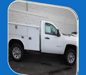
Traditional Bolt-on Service Body without pull-out drawer (45 cu. Ft.) Chevy w/XW9 Pickup Box Delete + spare tire.
